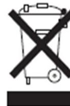
Do not dispose of SPH inverter together with household waste. Please accordance with the disposal regulations for electronic waste which apply at the installation site at that time. Ensure that the old unit and, where applicable, any accessories are disposed of in a proper manner.
